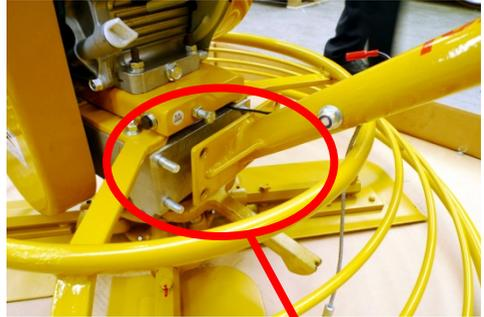
**STEP 4** – Remove the split-pin under the yoke lever. Insert the screwed end of the steel cable into the slot, with the nut behind the block and re-fit the split-pin. Bend the ends of the split-pin, so that it cannot fall out.
