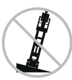
Do not depend on the tilt alarm as a level indicator. The tilt alarm sounds on the chassis only when the machine is on a slope.
