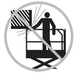
Be aware of crushing hazard when grasping the platform guard rail.
