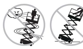
Do not drive the machine on or near uneven terrain, unstable surfaces or other hazardous conditions with the platform raised.
